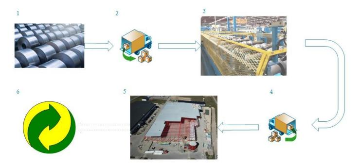
The steel coils (1) are produced at the steel manufacturer and transported to Lindab Profil Förslöv by truck (2). The high profile is produced in a roll forming machine (3). The production is a pull system (produced to customer order) to reduce waste in all parts of the life cycle. Transport to customers are done by truck (4) to the building site where the customer assemble the product (5). The usage phase is excluded in this EPD, it is why the next step is demolition and recycling (6).
